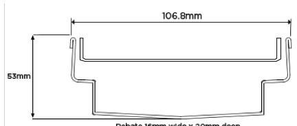
Grates longer than 1500mm supplied in sections. Tile Inserts longer than 1200mm supplied in sections. Channels over 3000mm supplied in sections with joiner. +/-2mm tolerance on dimensions.
