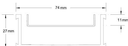
Grates longer than 1500mm supplied in sections. Tile Inserts longer than 1200mm supplied in sections. Channels over 3000mm supplied in sections with joiner. +/-2mm tolerance on dimensions.
