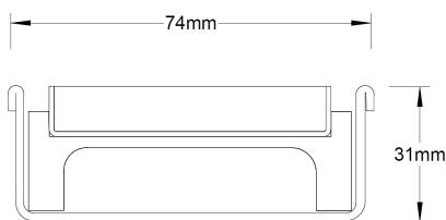
Grates longer than 1500mm supplied in sections. Tile Inserts longer than 1200mm supplied in sections. Channels over 3000mm supplied in sections with joiner. +/-2mm tolerance on dimensions.
