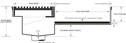
Grates longer than 1500mm supplied in sections. Tile Inserts longer than 1200mm supplied in sections. Channels over 3000mm supplied in sections with joiner. +/-2mm tolerance on dimensions.
