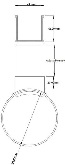
Grates longer than 1500mm supplied in sections. Tile Inserts longer than 1200mm supplied in sections. Channels over 3000mm supplied in sections with joiner. +/-2mm tolerance on dimensions.
