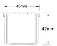
Grates longer than 1500mm supplied in sections. Tile Inserts longer than 1200mm supplied in sections. Channels over 3000mm supplied in sections with joiner. +/-2mm tolerance on dimensions.
